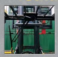
The Hyster® exclusive Vista masts widely spaced channels and overhead guard provide you with the industry's best all-around visibility for more confident load handling.
