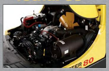
The engine cover, hinged at the rear, offers superior service access to the engine compartment with an opening angle of 85 degrees. The tough engine cover is made of a durable, crack-resistant, thermoset polyester resin reinforced with fiberglass.
