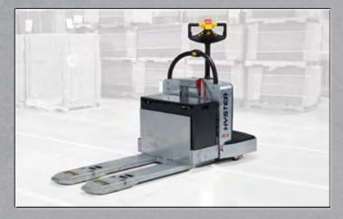
Hyster offers an optional Extreme Corrosion/Wash Down Package with a galvanized frame, lift linkage, battery well, and fork weldment. Where other lift trucks would rust and require additional cleaning and repainting, the B80ZAC with the Extreme Corrosion/Wash Down Package keeps on trucking. The galvanized frame pallet truck is designed for use in highly corrosive environments like food processing, pickling, tannery, chemical, salt and brine industries.
