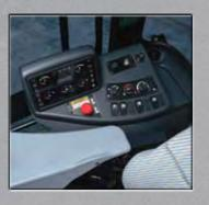
Diagnostics have been made simple with the state-of-the-art multi-function display panel which provides at-a-glance information via 16 warning lights, 5 gauges and dual function LCD.
