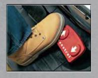
MONOTROL® Pedal- One foot control of acceleration and direction, leaving your hands free for steering and operating hydraulic levers. The Hyster MONOTROL® pedal helps keep your operators more productive.
