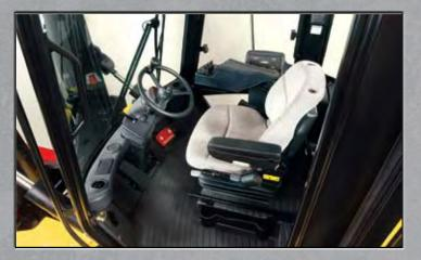
The ergonomic design of the cab and controls reduces operator fatigue and delivers improved productivity. The ComforCab II™ is large and uncluttered, allowing the operator ample room for auxiliary options. Operator compartment features a spacious environment with an adjustable suspension seat, with integrated armrest and low effort controls, 4-way adjustable steering wheel, and power-assisted steering and brakes. The cab's structural design creates excellent all-around visibility.
