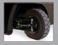
The elastomeric-mounted Hyster designed cast ductile iron steer axle with transverse, double-acting hydraulic cylinder, tapered roller spindle support bearings and non-adjustable tie rods provide maximum durability and superior steering control for easy maneuvering and low maintenance.
